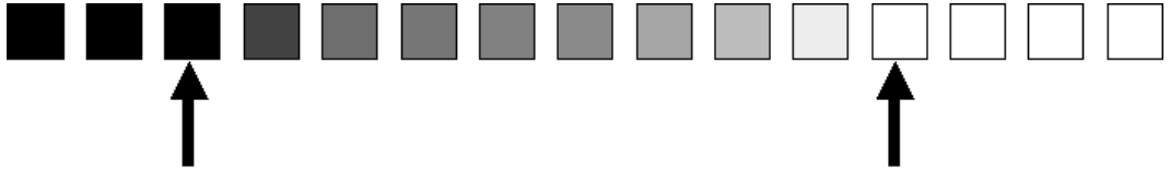
Figure 2.3: Illustration of a gradual shot change. The arrows indicate the start and end of the transition — ideally one would compare these two frames to detect a transition.
