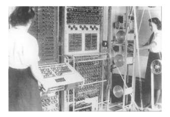
Figure 1. Colossus the first programmable computer.
