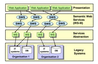
Fig. 3. A generic application architecture using IRS-III.
